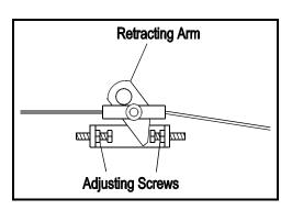
The final step is to ensure that the Track Parking Brake is functioning correctly. It is designed to stop and hold rated load on the stairway. To do this, the Brake Spring must pull on the Brake Mechanism without any resistance from the Brake Cable. This can happen if the Front Brake Cable does not have sufficient slack.
