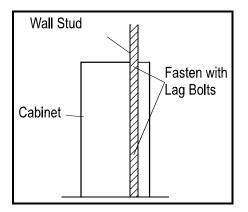
To attach to concrete or to a concrete block wall, drill three 8 mm (5/16 in) diameter holes as shown in the back of the cabinet. Position the cabinet against the wall and, using the drilled holes as a guide, drill three holes in the wall. The size of the holes will depend on the type of insert or plug being used. Insert suitable plugs and fasten the cabinet to the wall using lag bolts.
