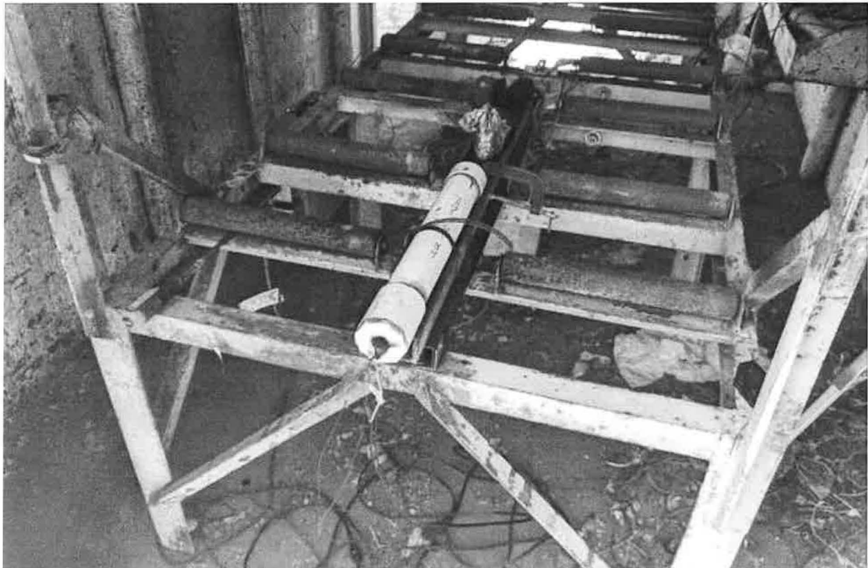
Fig 2: Mason's fabricated experimental ANCP motor on the test stand.
