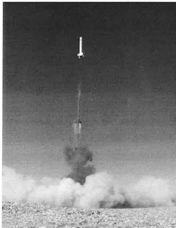
Fig 15: Booster accelerates at 120g off the launch rail
