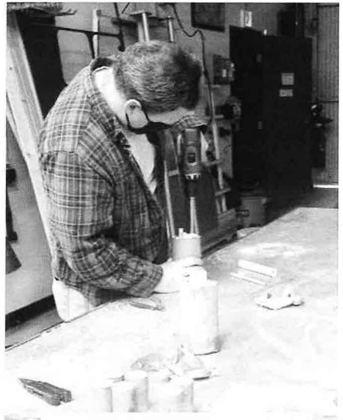
FIG 2: Preparing finocyl grains
