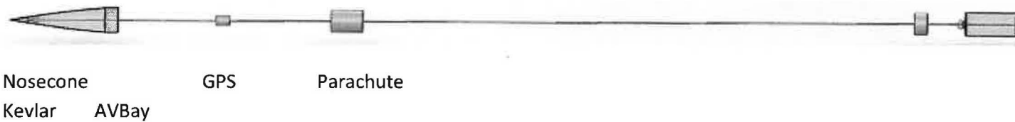
Figure: Forward recovery layout to accurate scale.
