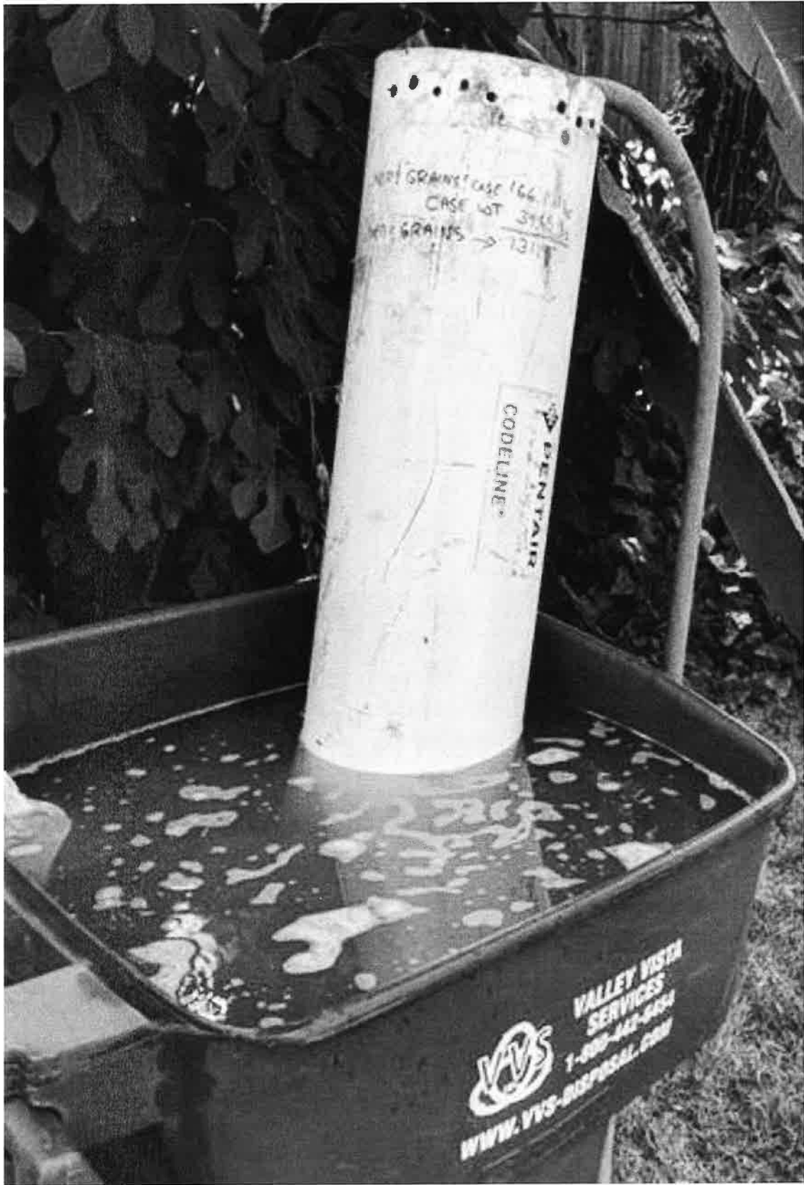
Fig 6: Prepping a motor to fire again after test fire. The wonder of a water soluble propellant.
