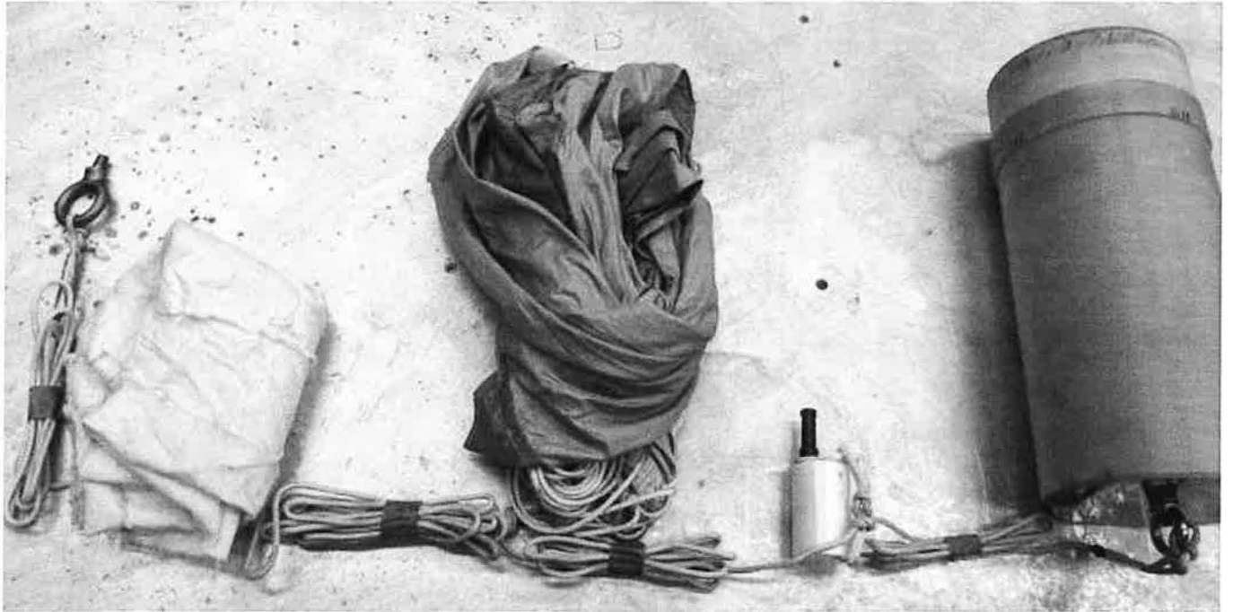
Step 14: Layout main recovery materials from left to right including 3/8" motor mount eyebolt, nomex blanket, 72" parachute, GPS module and 8mm eyenut.
