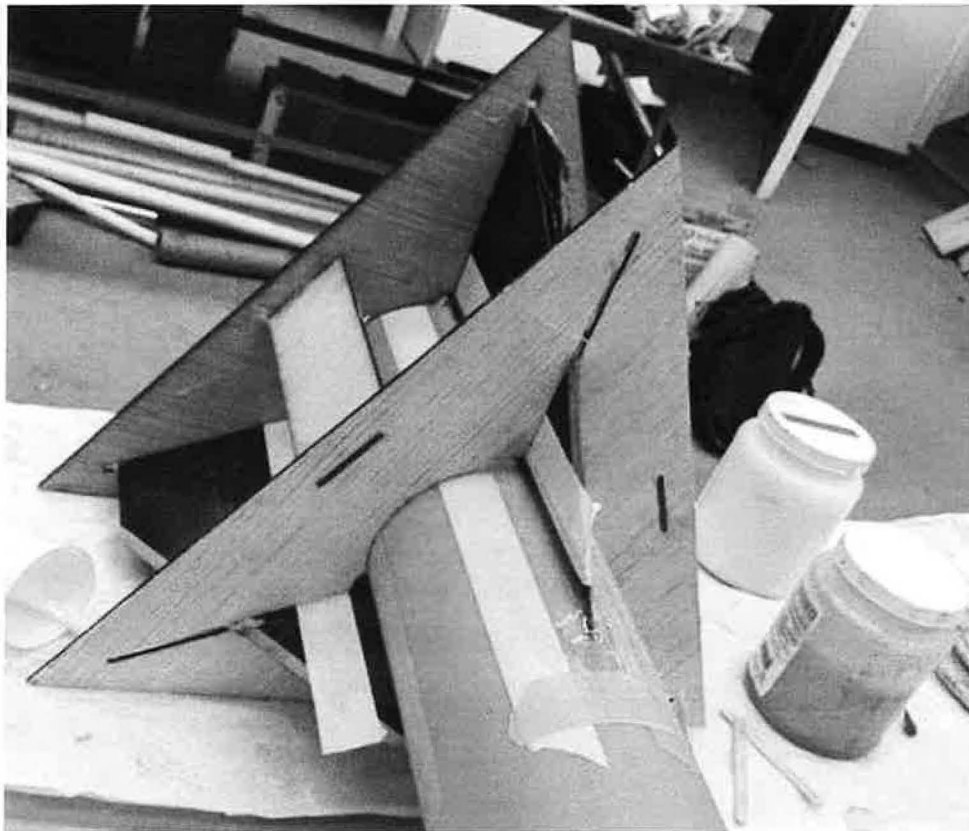
Step 6: Assemble fins and layup epoxy fillets.
