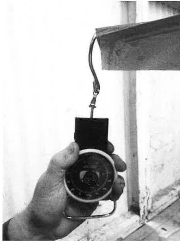
Fig 3: Deflection testing the fins
