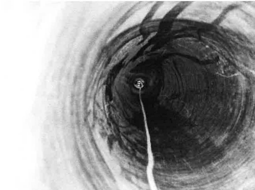
Step 11: Install ¼-20 eyebolt into aluminum tip of nosecone.
