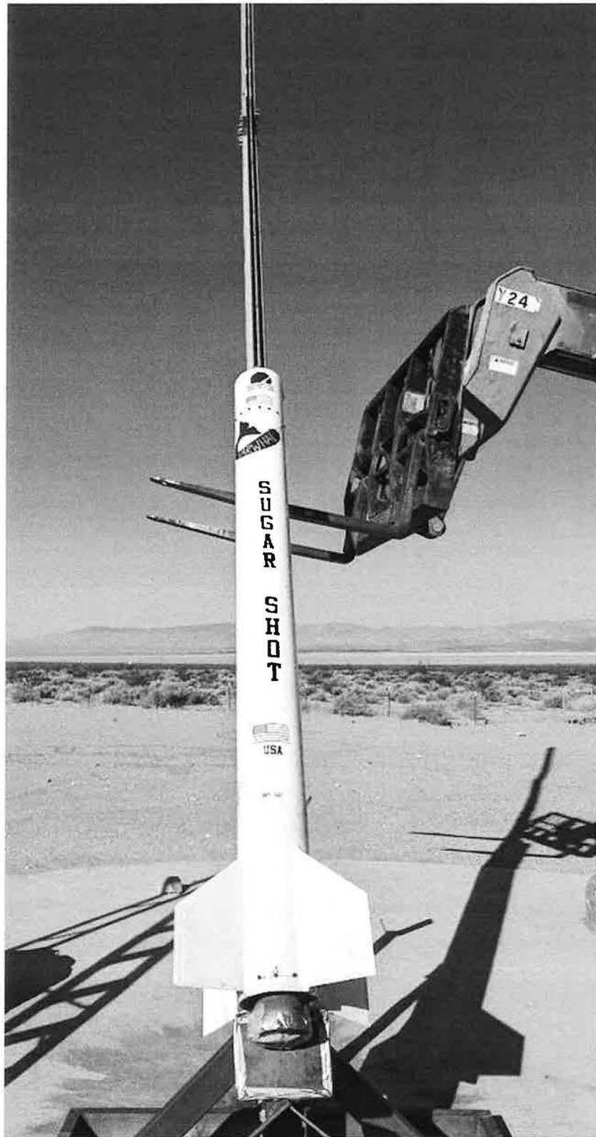
Fig 13: Lifting the booster up on the rail
