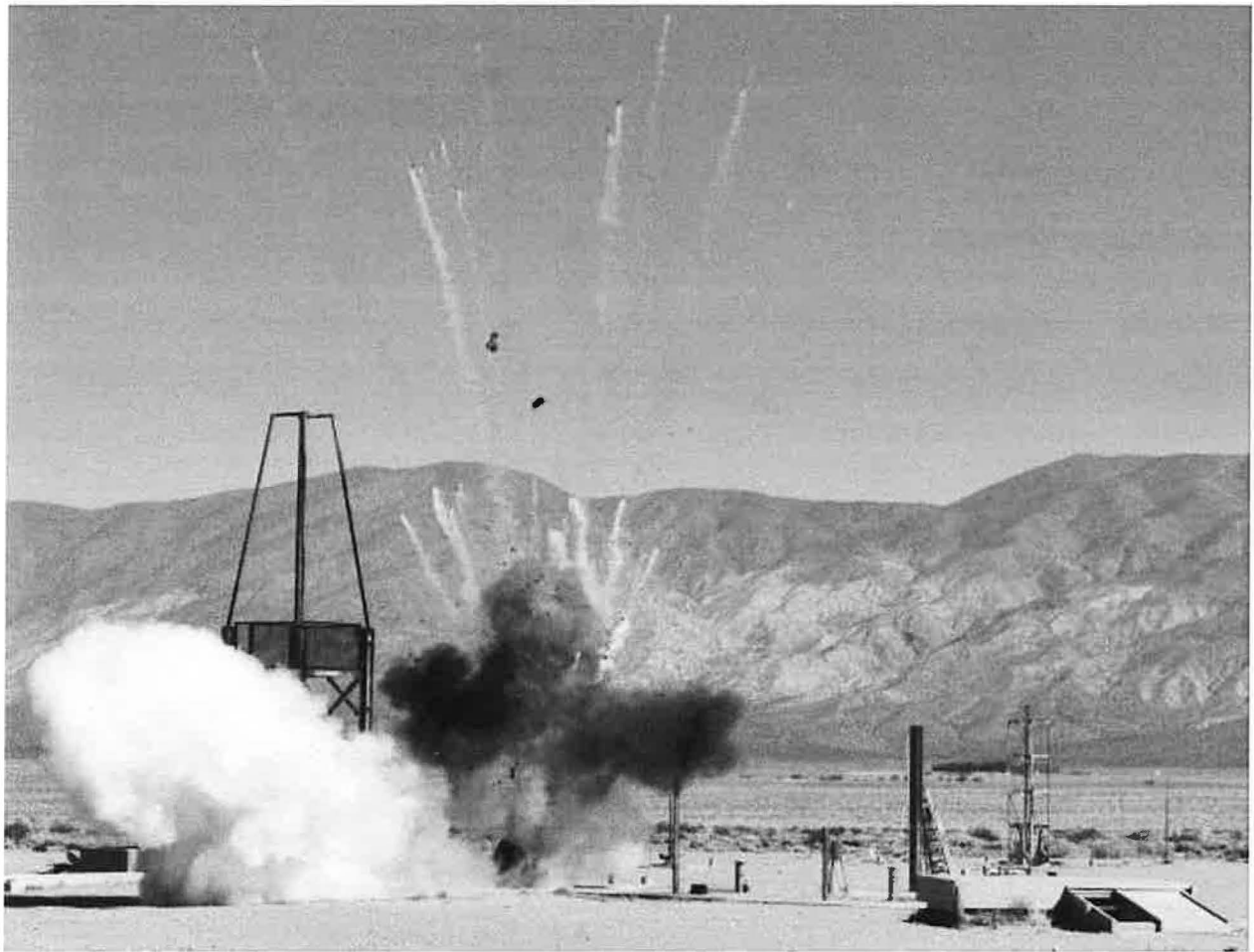
FIG 11: Static Motor failure
