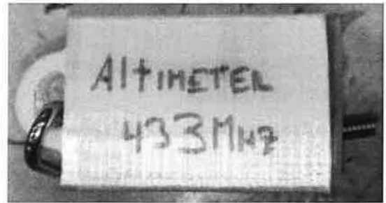
FIG 2: TPU case for SS2S Avionics Board
