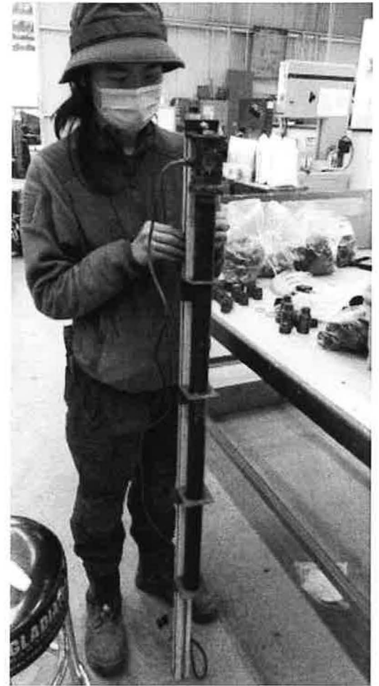
FIG 1: Fabricated motor with custom test stand and load cell
