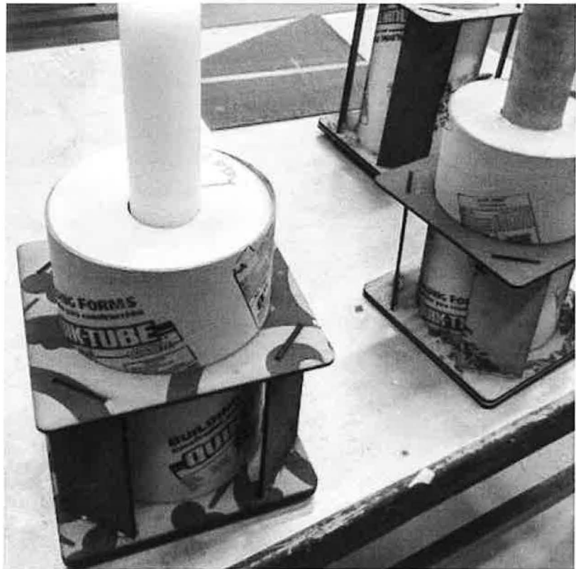
FIG 7: Grain casting jig
