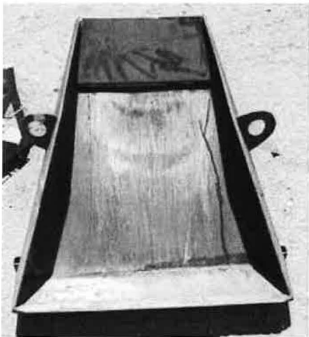
FIG 2 Repaired flame bucket
