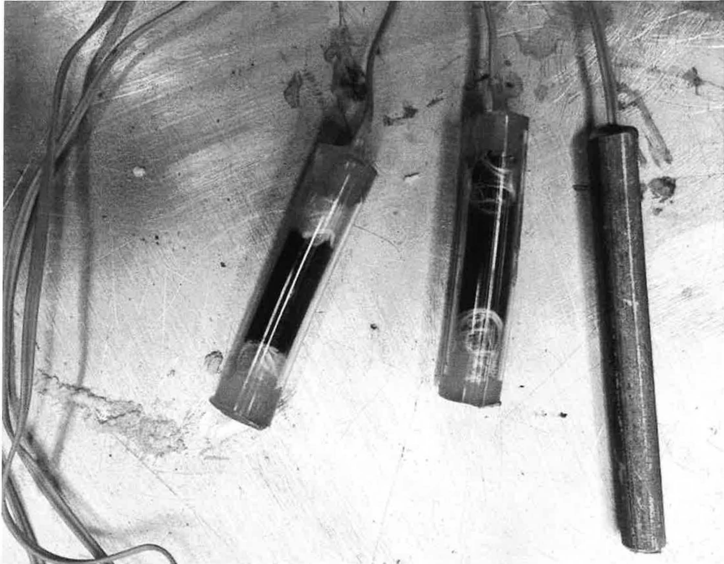
Step 17: Fabricate ejection charges. Two left charges are 1 gram black powder in vinyl tubes sealed with hotglue. The right tube is an backup 1 gram Jim Jarvis style high pressure ejection charge.
