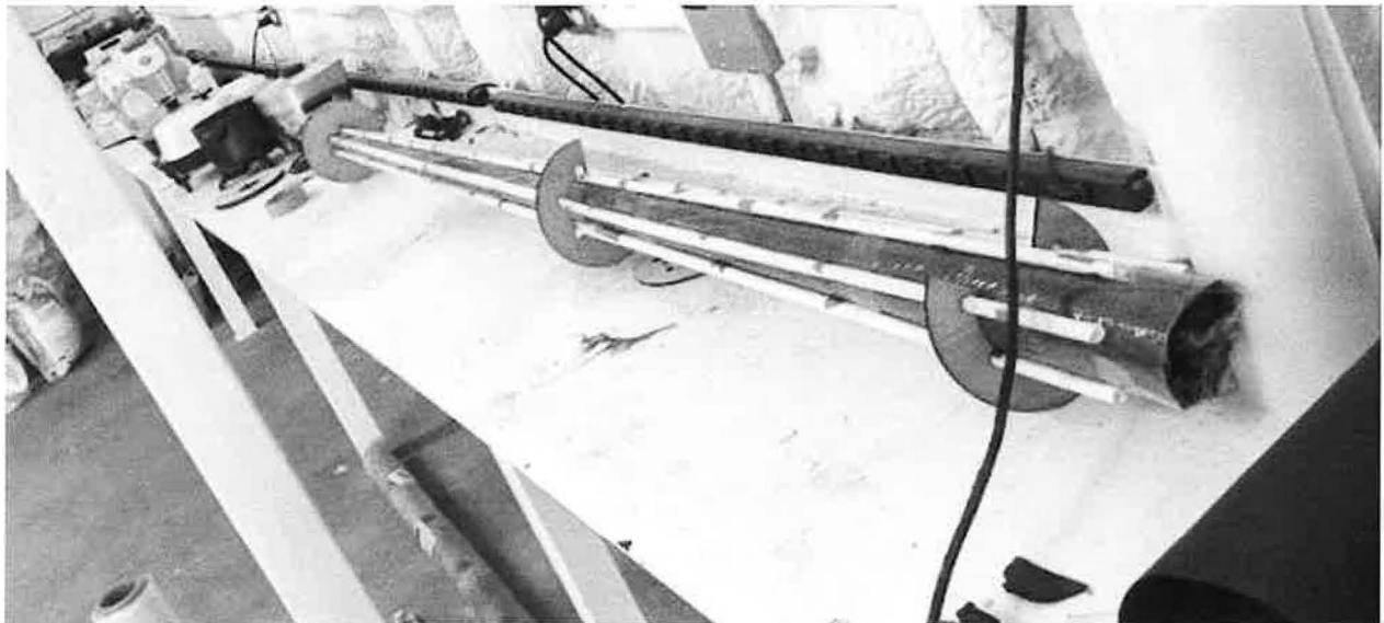
Fig 9: Finocyl assembly wrapped in polyethelene
