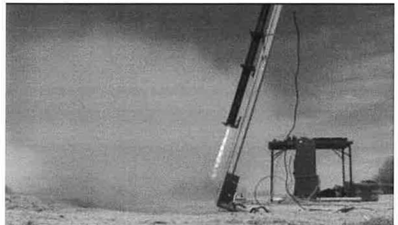
FIG 2: Successful test fire of hybrid motor with mach diamonds
