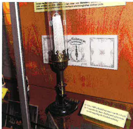
Original Bunsen burner, fitted with mantle.
